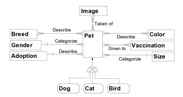
There is more than one way to create a conceptual data model in ER/Studio. The animal shelter chose the approach of hiding the attributes (under "Diagram And Object Display Options", select "Display Level" of "Entity").
