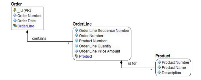
Notice the containment line with the black diamond. This shows that OrderLine is contained in Order, and Product is contained in OrderLine. The tool has created an array field with the same name as the object OrderLine. This view is quite useful to see how nested objects repeated in multiple parents are used.
