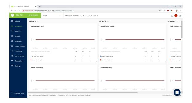
SQL Diagnostic Manager for MySQL contains 600 out-of-the-box monitors, including many for Galera Cluster. Each monitor has a current status for the selected nodes; here, the three nodes in the Galera Cluster. Moving the mouse cursor over the monitor shows a description of what that monitor is measuring.
