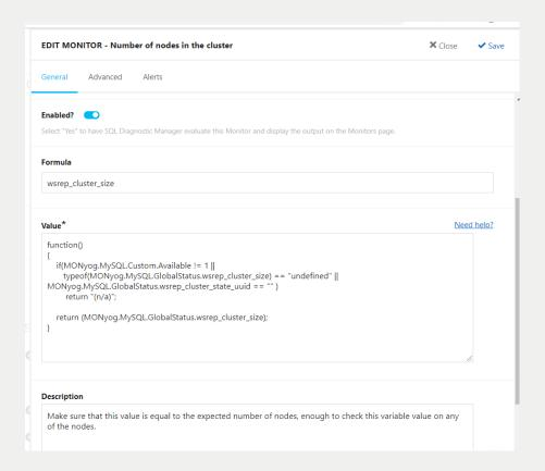
The 'Alert Condition' JavaScript function allows customizing the code that determines the status of each monitor. It will be alright, near-critical, or critical.
